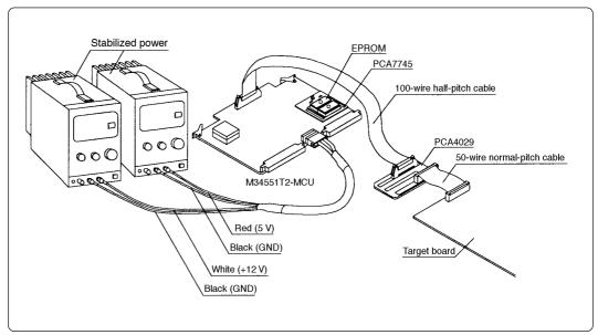
Figure 5.1 System configuration for using as evaluation board
